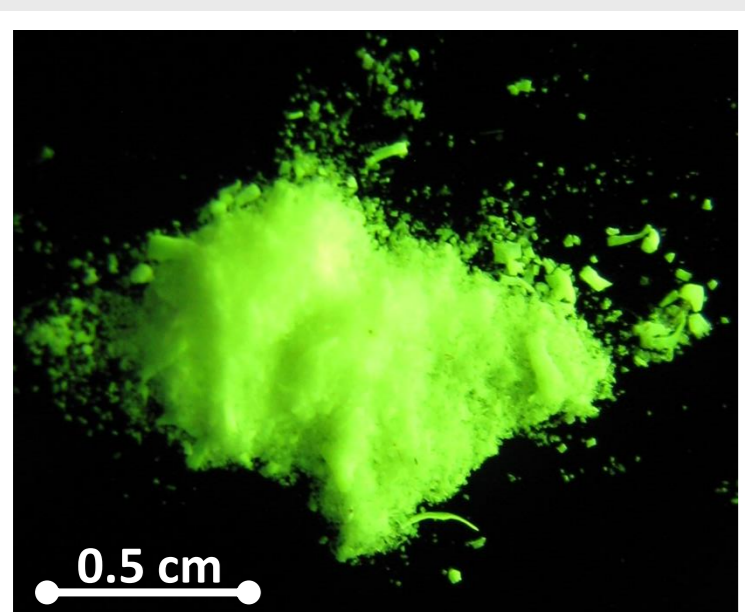
NP-powder of CaF 2 :Tb 3+ ,Gd 3+ -NPs under excitation with UV-lamp (λ ex = 254 nm)
